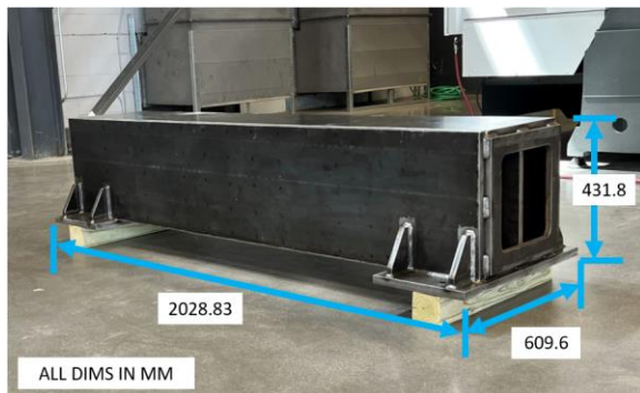
FIGURE 2. Identical cross beam weldment that is from the concrete base machine tool.
