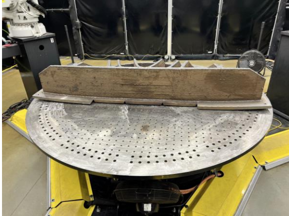
FIGURE 8. Front face of the mBAAM cross beam at the end of the print.
