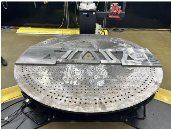
FIGURE 5. MedUSA build table with five separate build plates before implementing steel clamps.
