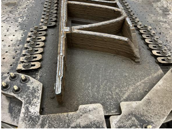
FIGURE 11. Print beads on the mBAAM part along the long axis could have contributed to the uneven thermal gradient of the print.
