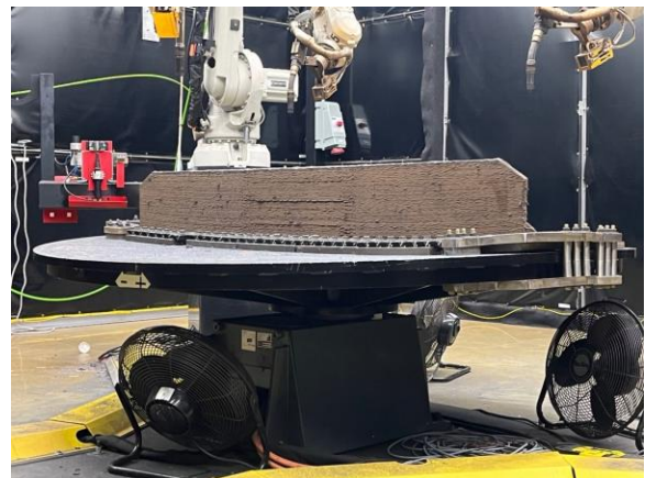
FIGURE 7. Deformed mBAAM cross beam and build table.
