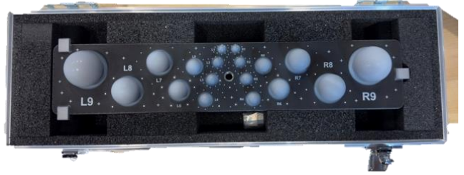
FIGURE 5. ZEISS PSA 400 artifact used for performance evaluation.
