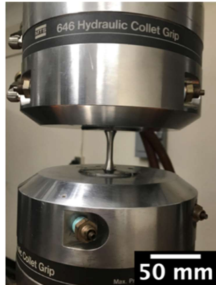
Fig. 4. Servo-hydraulic test frame and grip setup for uniaxial HCF tests.
