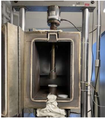
Fig. 2. MTS servo-hydraulic press with furnace chamber for isothermal hot forging. Specimens were compressed on a single axis.
