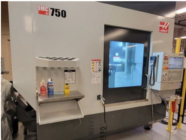
Fig. 3. HAAS UMC-750 5-axis machining center. The pneumatic entry door is partially in view, looking through the front door window.
