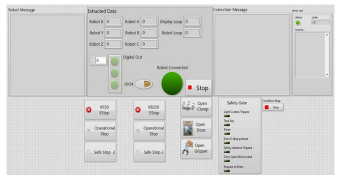
Fig. 6. LabVIEW operator interface for monitoring and controlling the hybrid manufacturing cell.
