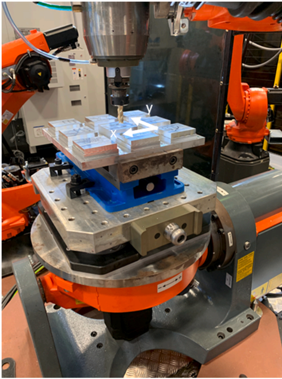
Fig. 7. Setup for workpiece mounted in a vise attached to the top axis (rotation about z axis) of the rotary positioner. The x and y machining directions are identified and the tool-holder-spindle attached to the robot end effector is shown.
