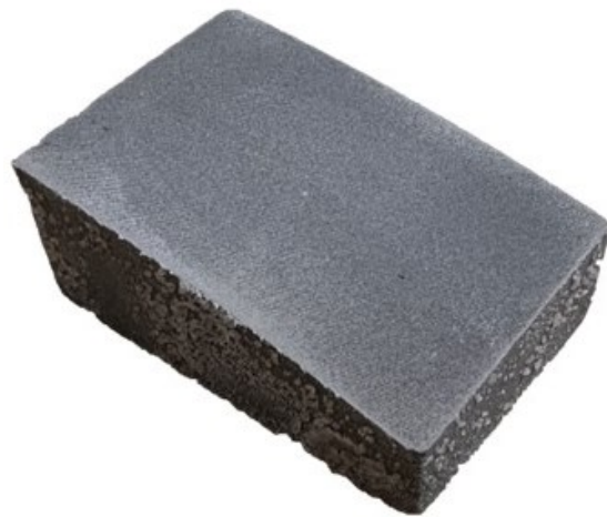
Figure 8. Machined BJAM SiC sample.
