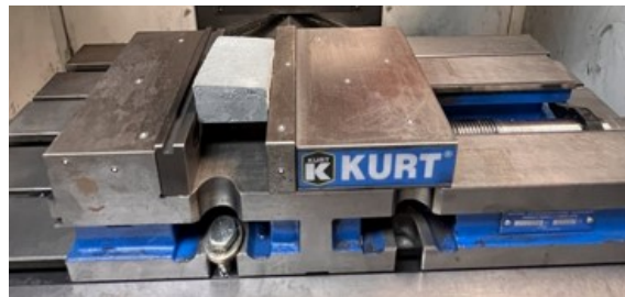
Figure 4. Infiltrated sample clamped in milling machine vise on machine table [19].
