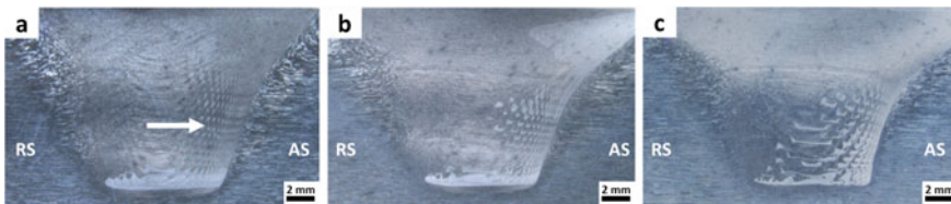
Fig. 2 Macrostructure of the processed materials fabricated at different tool rotation speeds of a 400 rpm, b 600 rpm, and c 800 rpm showing a difference in materials flow lines at steady-state processing conditions
