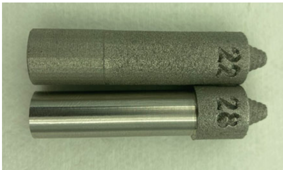
Fig. 1 Image depicting the two tools, tool 28 which has been turned down and tool 22 which has not
