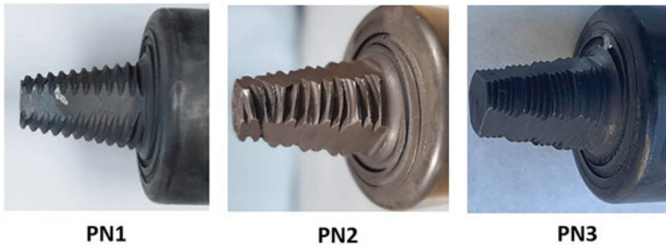
Fig. 2 Left: Base tool used in this study referred as PN1. Center: First iteration of opposing thread tooling PN2. Right: PN3 tool containing opposing/finer thread. PN1 and PN3 are compared in the Results and Discussion
