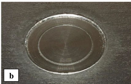
Fig. 2 a RFSSW tool set consisting of clamp, shoulder, and probe (from left to right). b Refill friction stir spot weld in aluminum sheet. c Bond Technologies refill friction stir spot welding end effector
