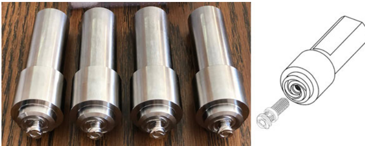
Fig. 1 Example set of preproduction SBT toolsets. Each tool is comprised of (1) the SBT probe and (2) the tool body with integral shoulder [16]
