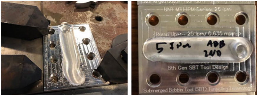
Fig. 16 First set of SBT test coupons processed on the UNT robotic FSP system: before positioning compensation (left) and after compensation (right). The travel speed was 127 mm/min, and the rotational rate was 750 rpm for both coupons
