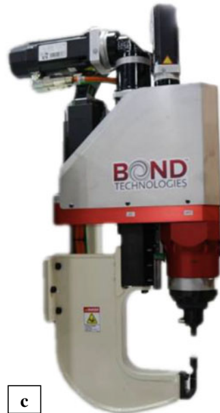
Fig. 2 a RFSSW tool set consisting of clamp, shoulder, and probe (from left to right). b Refill friction stir spot weld in aluminum sheet. c Bond Technologies refill friction stir spot welding end effector
