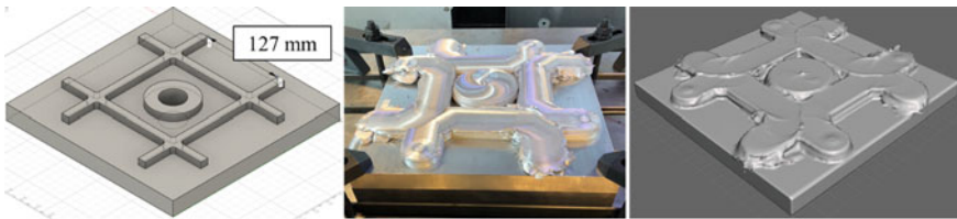
Fig. 2 (Left) CAD model of panel. (Middle) 6061 aluminum preform. (Right) scanned preform model
