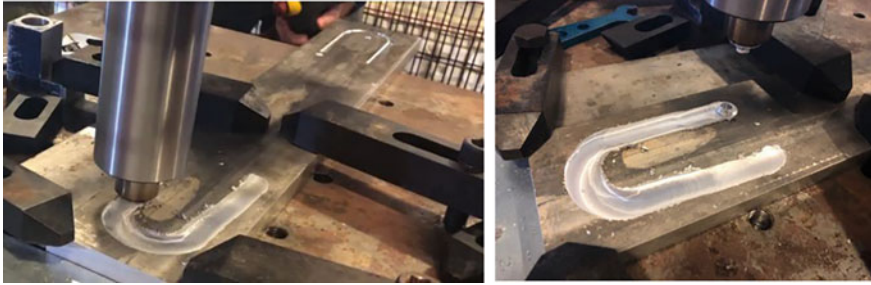
Fig. 19 Second U-shaped channel processed on the UNT robotic FSP system at 127 mm/min and 750 rpm. This process run included side-deflection correction
