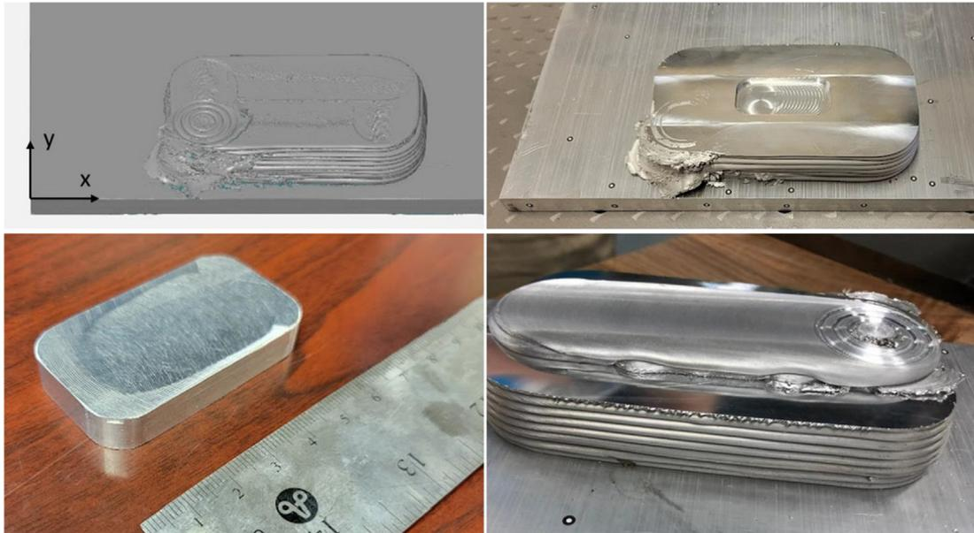
**Fig. 2.** Manufacturing sequence for embedding QR tag (clockwise from top left). (Top left) The AFSD part was scanned to identify the stock model for the first machining operation. (Top right) The top surface was faced and the pocket was machined to hold the QR tag. (Bottom right) Additional layers were deposited over the QR tag. (Bottom left) A coupon was obtained for CT scanning by machining material away with a 3 mm perimeter around the embedded QR tag.
