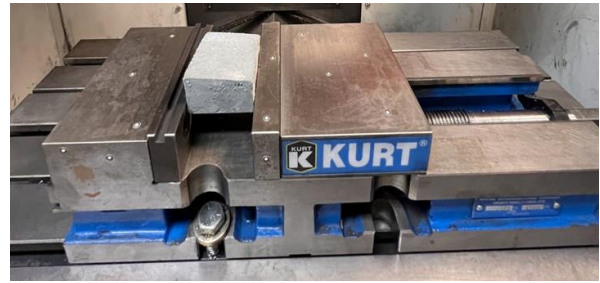
FIGURE 4. Infiltrated sample clamped in milling machine vise.
