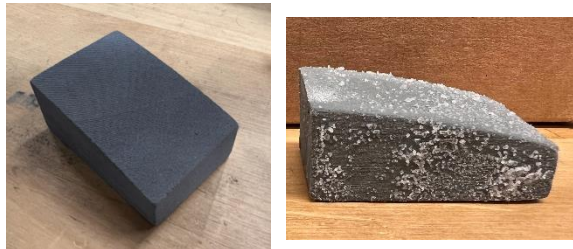
FIGURE 3. Silicon carbide sample as printed from BJAM (left) and after infiltration (right).
