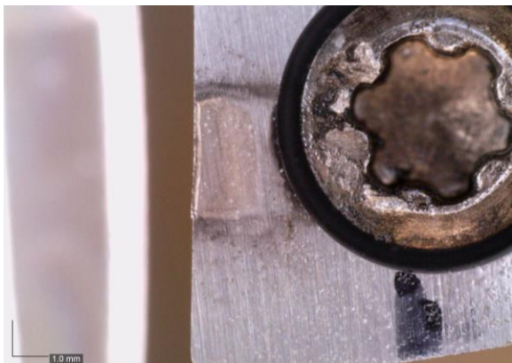
FIGURE 10. 28.3x image of the insert 6 rake face after the first test cut.
