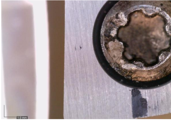
FIGURE 9. 28.3x image of the insert 6 rake face prior to initial test cut.
