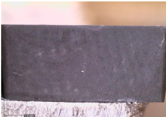
FIGURE 11. 46.4x image of the insert 1 flank face prior to the initial test cut.
