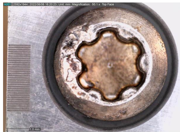
FIGURE 13. 50.1x image of the insert 1 rake face prior to initial test cut.
