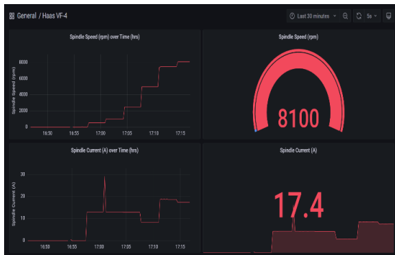
FIGURE 9. Grafana dashboard displaying spindle speed and spindle current over a period of 6 hours.
