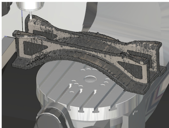
Figure 12: Simulation for feet machining
