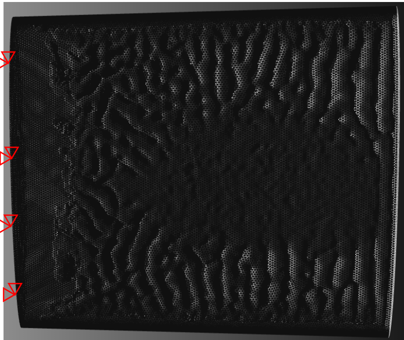
Figure 5. Resulting optimized geometry for the ellipsoid, looking down on the loaded face. The fixed displacement constraints of the geometry are represented on the left end.
