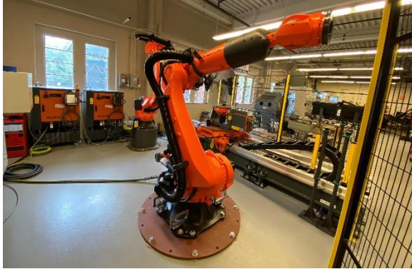
FIGURE 5. KUKA KR250 industrial robot for moving parts between the linear track and the machining center.
