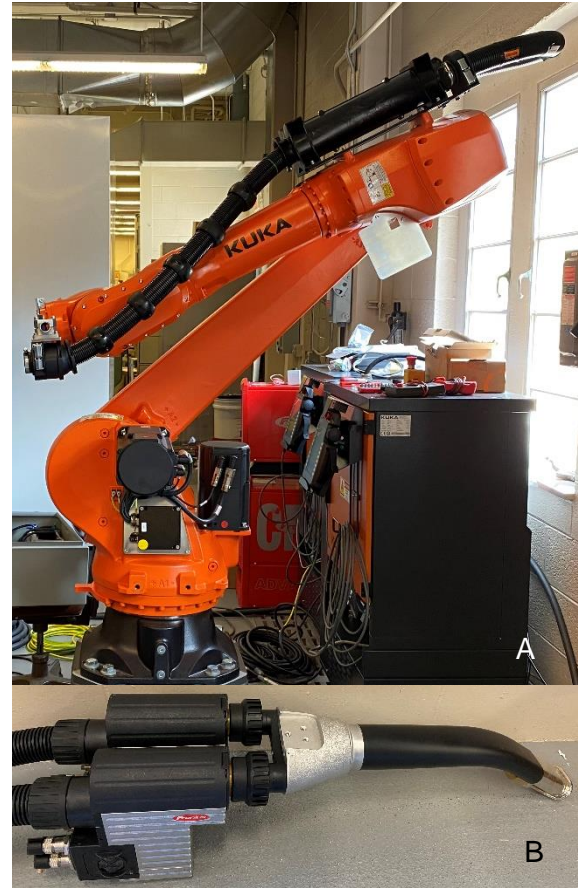
FIGURE 2. (A) KUKA KR50 industrial robot used for WAAM process (B) Dual wire CMT Advanced welding torch.
