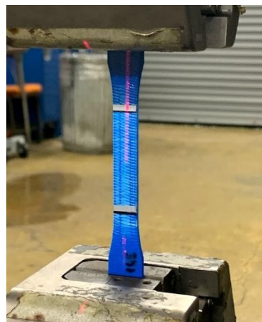
FIGURE 1. Tensile test experimental setup. The ABS specimen is clamped in the universal testing machine.
