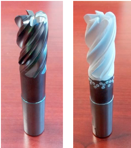
Fig. 1. Tool preparation for structured light scanning. (Left) variable pitch endmill. (Right) application of i -PrOH \text{TiO}_2 coating and reference targets.
