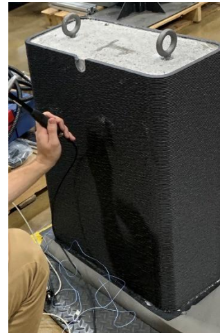
FIGURE 3. Section of mold removed to allow for direct measurement on concrete.
