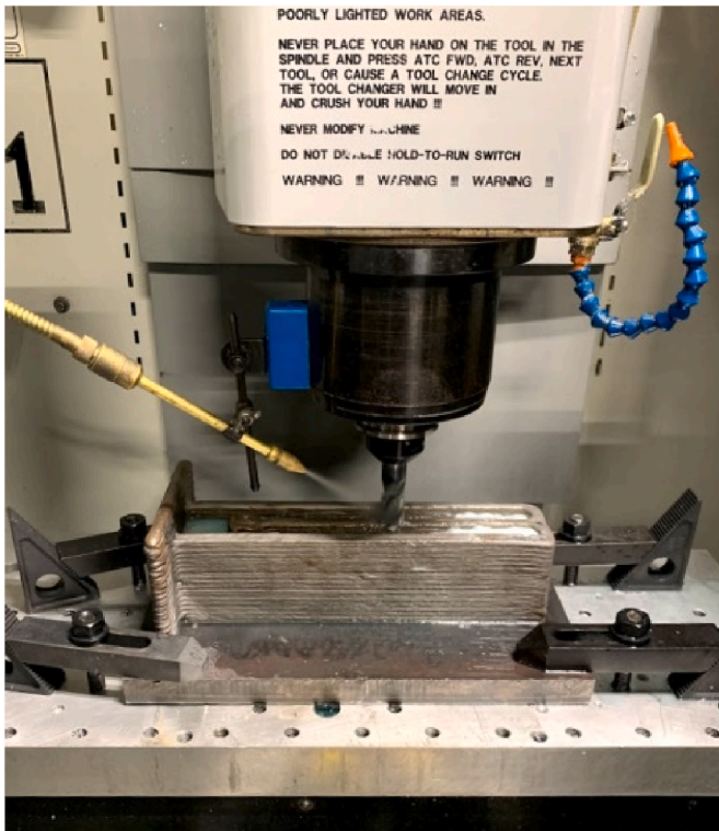
Fig. 8. To machine the first side, the build plate was clamped to the machine table. The top surface was then faced.
