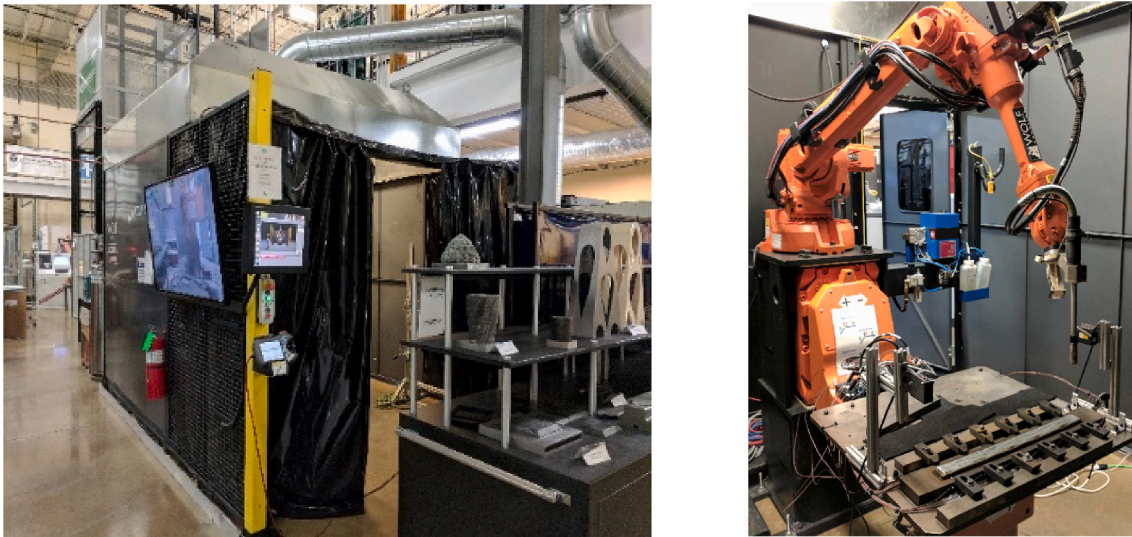
Fig. 5. (Left) External protective walls for the mBAAM system. (Right) The deposition head located above the printing position.
