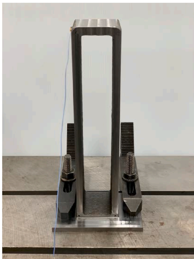
Fig. 11. Impact testing was used to measure the final part FRFs. For the FRF measurements, the parts were clamped to a rigid table to approximate fixed-free boundary conditions. A low-mass accelerometer is shown attached to the top right of the part.
