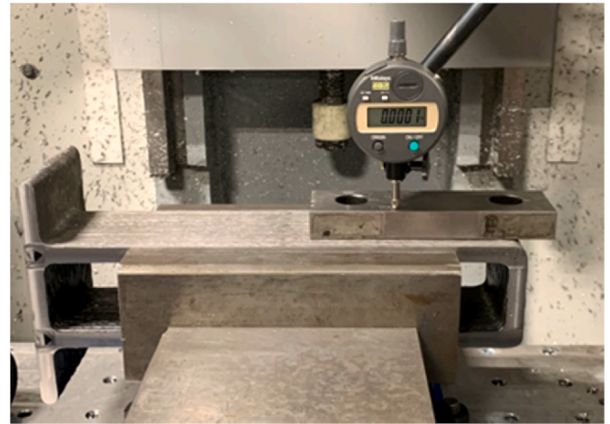
Fig. 9. The parts were clamped in a vise and a machining parallel was used as an indicating surface for the dial indicator to align the part.
