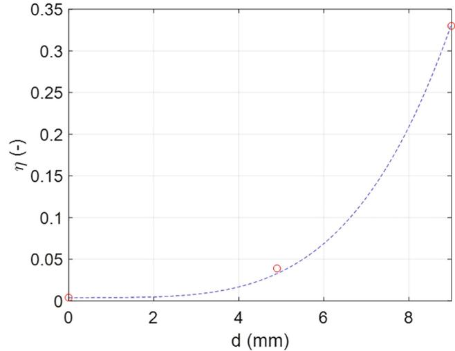
**Fig. 9.** Damping factor data (circles) and fit (dashed line) versus inner diameter.
