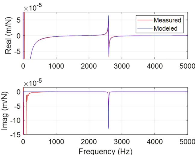
**Fig. 6.** Measured and modeled FRF for solid cross-section cylinder.
