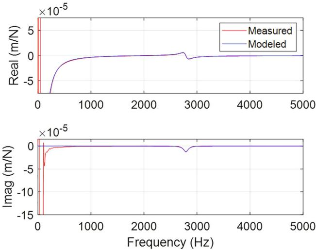
**Fig. 8.** Measured and modeled FRF for hollow cross-section cylinder with captured powder (4.9 mm inner diameter).
