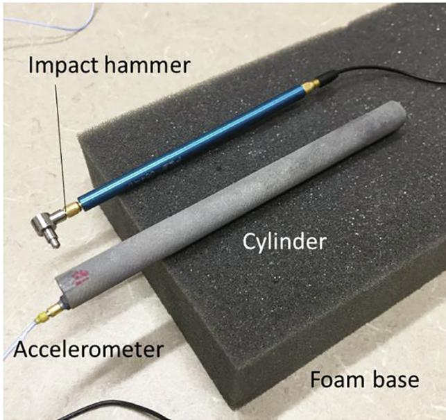
Fig. 1. Impact testing setup for FRF measurement.
