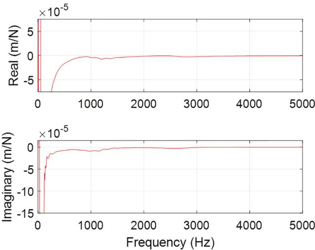
**Fig. 5.** FRF for hollow cross-section cylinder with captured powder (9.0 mm inner diameter).
