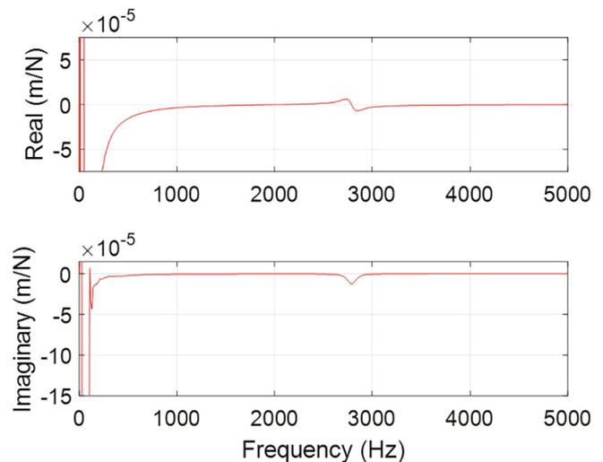
Fig. 3. FRF for hollow cross-section cylinder with captured powder (4.9 mm inner diameter).
