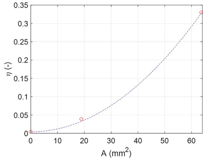
**Fig. 10.** Damping factor data and fit versus inner cross-sectional area.
