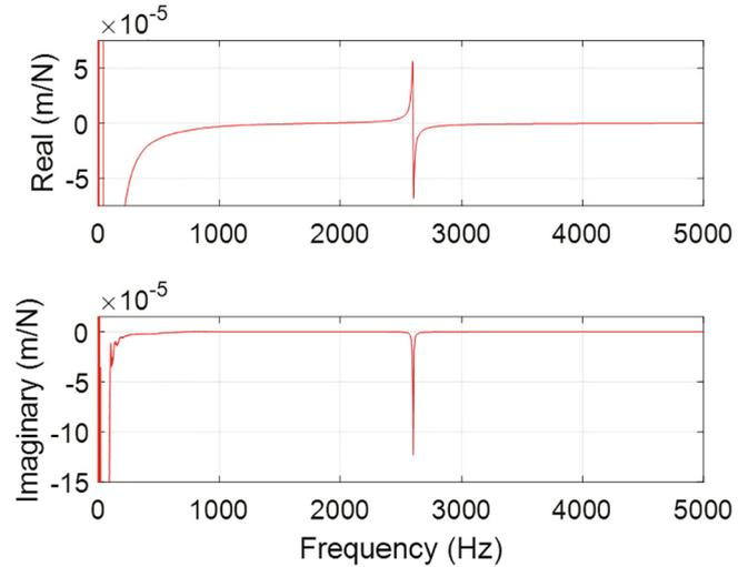
Fig. 2. FRF for solid cross-section cylinder. (Top) Real part. (Bottom) Imaginary part.
