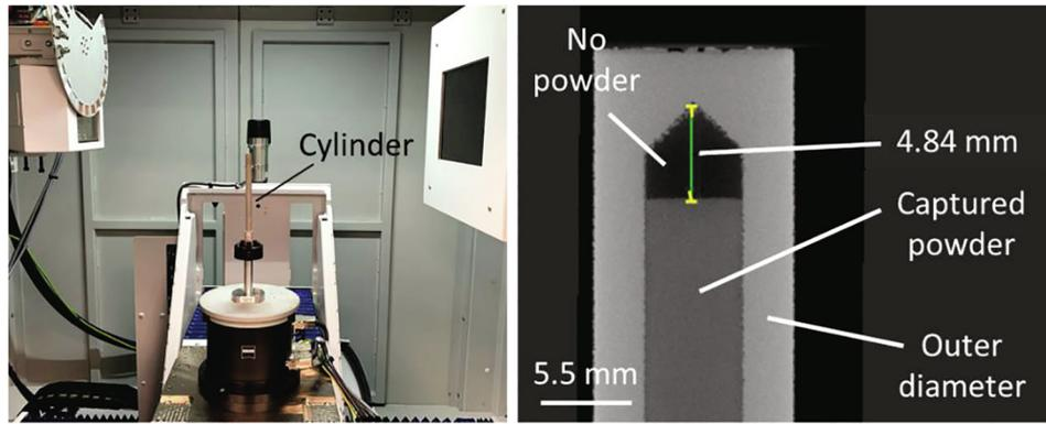
**Fig. 4.** (Left) CT setup for vertical cylinder measurement. (Right) Example measurement result for 4.9 mm inner diameter cylinder. The density difference between the sintered outer diameter (light) and captured powder (dark) is identified by the image gray scale. No significant porosity is observed in the outer diameter and the incomplete powder fill is seen (i.e., the black section above the captured powder).
