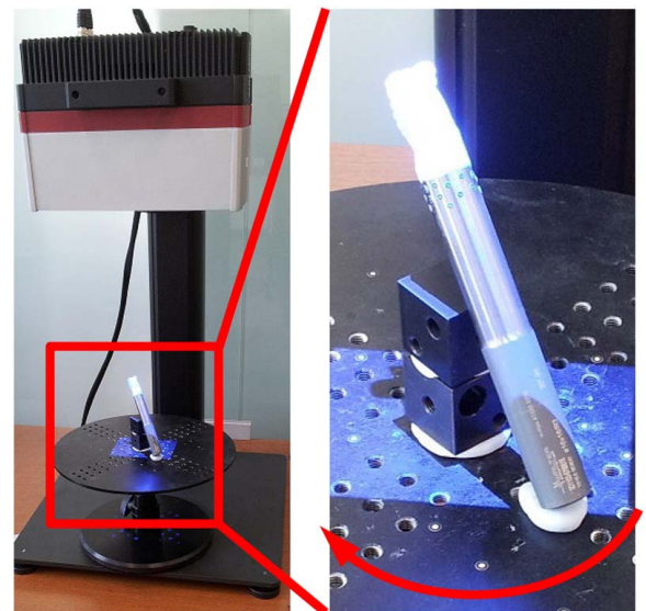
Fig. 2 Scanning metrology setup using the GOM ATOS Capsule system
