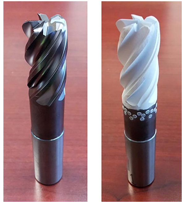
Fig. 1 Endmill preparation for structured light scanning: example endmill (left) and application of anti-glare coating and reference targets (right)
