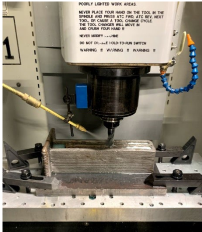
Figure 8: To machine the first side, the build plate was clamped to the machine table. The top surface was then faced.
