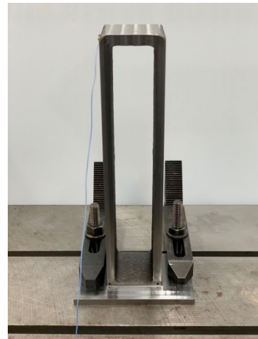
Figure 11: Impact testing was used to measure the final part FRFs.
