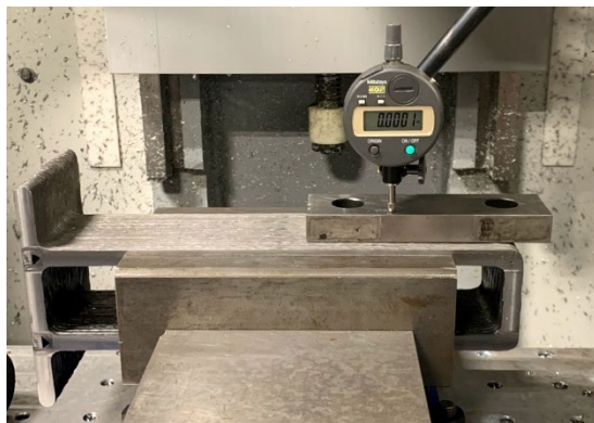
Figure 9: The parts were clamped in a vise and a machining parallel was used as an indicating surface for the dial indicator.
