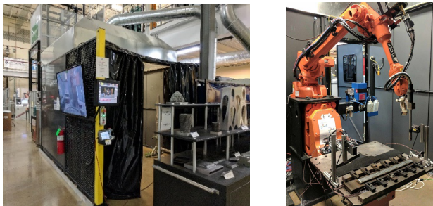
Figure 5. mBAAM system. (Left) external protective walls. (Right) deposition head over printing position.
