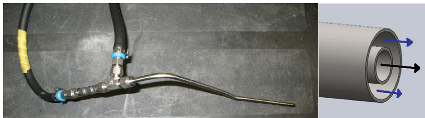
Fig. 2. Gas delivery system. The inner tube supplied the acetylene gas. The outer annular tube provided the nitrogen gas shield.
