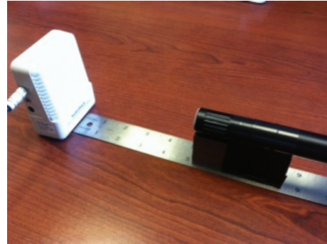
FIGURE 3: Experimental setup. The speaker is on the left and the unidirectional microphone is on the right. The distance between them is determined using the steel scale.
