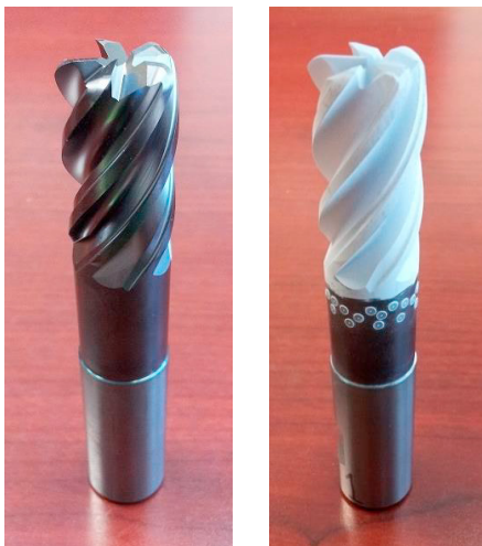
Fig. 1. Tool preparation for structured light scanning. (Left) example tool. (Right) application of i -PrOH TiO 2 coating and reference targets.
