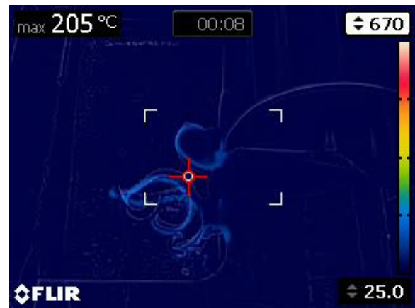
FIGURE 11. Thermal image showing maximum cutting temperature for the MTP feed turning operation.
