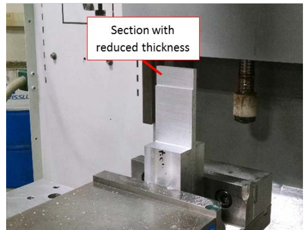
Fig. 5. Experimental setup. (Top) The fixed-free aluminum beam was mounted in a vise which was clamped to the machine table. The laser vibrometer was used to measure the beam response due to a force impact (applied by a modal hammer). (Bottom) The beam thickness was reduced over a section with a known length and receptance measurements were performed at the top and bottom of the section.
