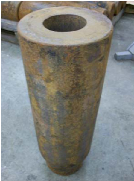
Fig. 2. Photograph of typical extrusion. The length is 520.7 mm and the mass is 76 kg.
