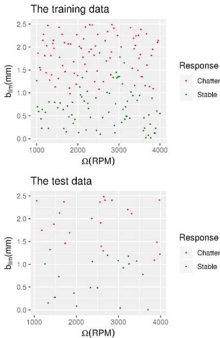
Fig. 10. The data used for training (top) and testing (bottom) the neural network model.
