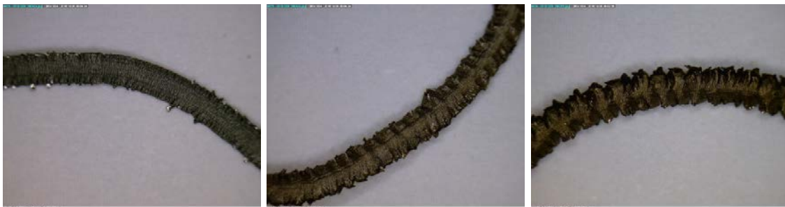
Fig. 17. Microscope images (50x) for constant feed rate tests ( \Omega = 168 rpm, v_c = 37.5 m/min): (left) f_r = 0.102 mm/rev; (middle) f_r = 0.152 mm/rev; and (right) f_r = 0.203 mm/rev.
