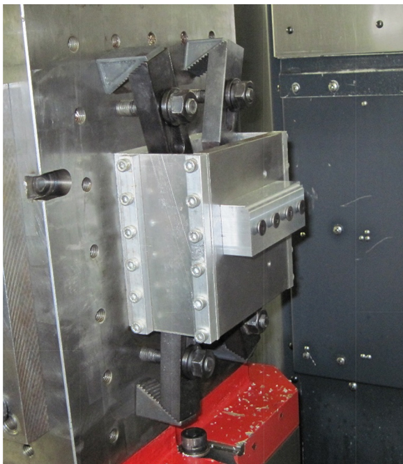
Fig. 11. Setup for validation testing. The parallelogram type flexure and attached workpiece are mounted to the machine tool’s tombstone.
