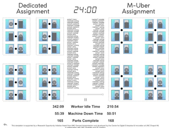
Figure 4: Simulation software that compares the traditional (dedicated) and M-Uber assignment techniques.
