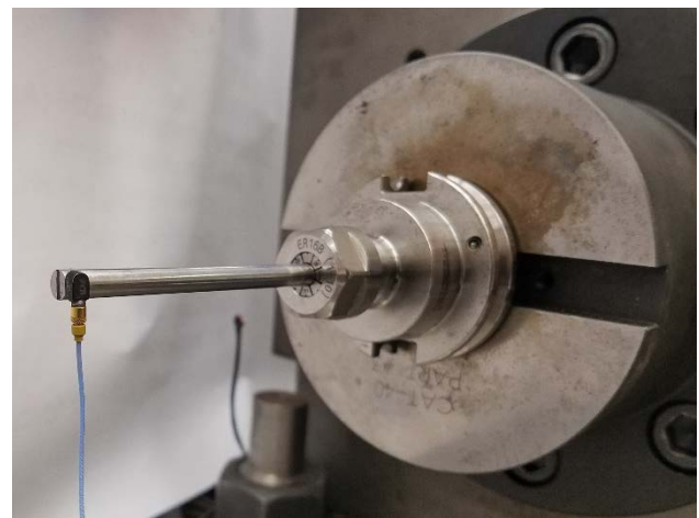
Figure 8. Small accelerometer attached to the 6.35 mm diameter rod using modal wax.
