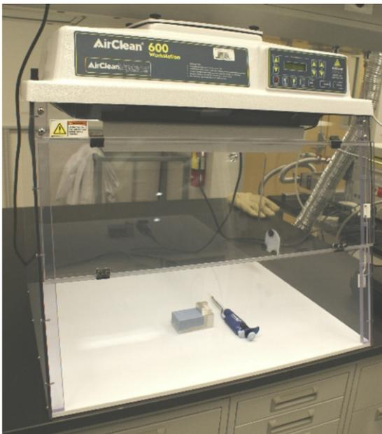
Fig. 7. All samples were bonded in a class 100 laminar flow clean cube to avoid including airborne particles in the bonded interface.
