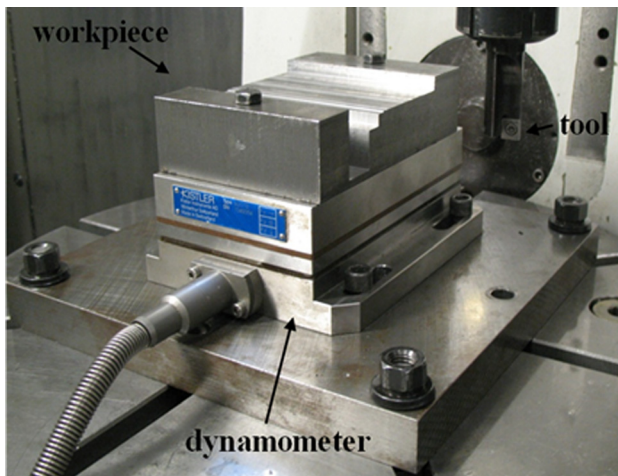
Fig. 8 Experimental setup for milling force measurement
