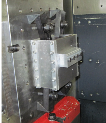
Figure 5. Setup for validation testing. The parallelogram type flexure and attached workpiece are mounted to the machine tool's tombstone.
