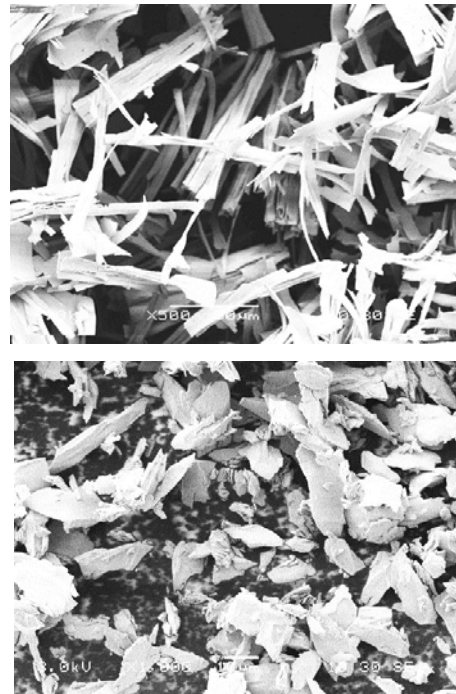
FIGURE 4. Chip morphology at 800X for (top) h = 400 \text{ nm} and (bottom) h = 1.4 \mu\text{m} .
