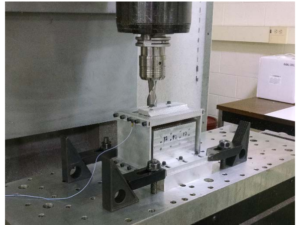
Figure 6: Milling setup showing damped flexure, two-flute endmill, and accelerometer.
