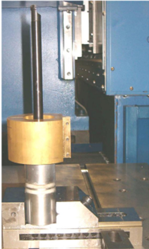
Fig. 10. Set-up for frequency response measurements of the vise–holder–sleeve–boring bar assembly.
