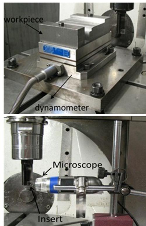
Fig. 1 Dynamometer/workpiece (top) and microscope for in process measurement of  $F_{WW}$  (bottom)
