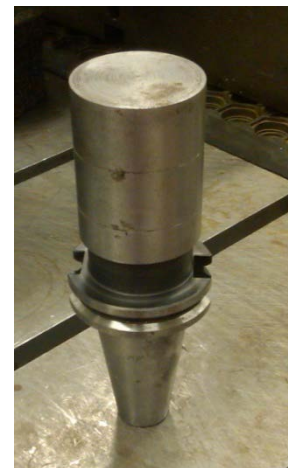
FIGURE 2. Standard holder used to measure spindle-machine FRF (CAT-40 interface).
