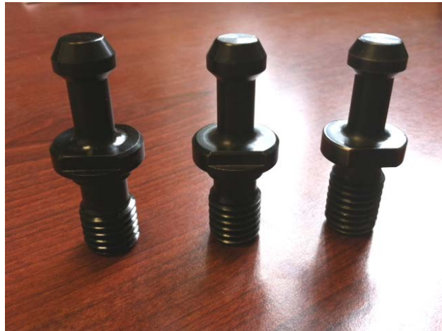
Figure 2. Three retention knobs: (left) restricted thread length design A; (middle) restricted thread length design B; and (right) traditional design C.
