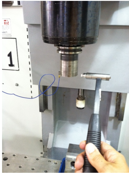
Figure 1. Photograph of modified boring bar (artifact) mounted in the CAT-40 spindle interface; the retention knob cannot be seen. The accelerometer and hammer are also shown for an x direction measurement.
