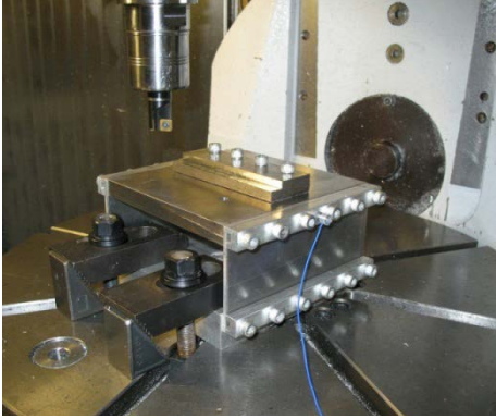
Figure 11. Setup for milling stability tests. An accelerometer was used to measure the vibration signal during cutting.
