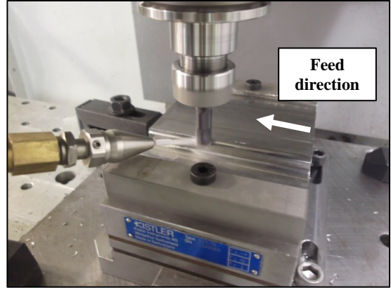
Figure 1. Milling setup using a cutting force dynamometer.
