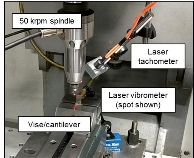
Figure 5. Experimental setup. The rib was machined to reduce the thickness and the receptance was measured for multiple L_2 values.
